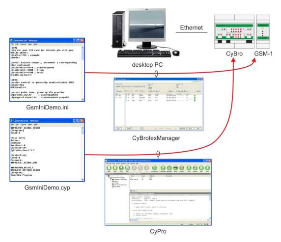
After transfer is complete, module will reset automatically. Minute or two later, it will connect to network, and both GSM and GPRS LEDs will be green. If configuration file has errors, GSM LED will blink.
