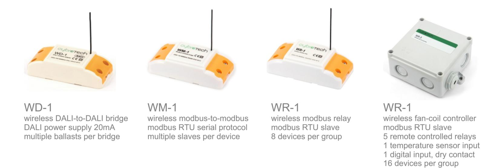
Common features: very long range, no hopping, protected private connection, multiple addressable groups. The operating range is 300-500m with no obstacles. Cybro with RFM option can control any of the modules.
